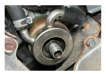
7. Lubricate the sandwich plate o-ring using new engine oil. Install the sandwich plate centre bolt finger tight then 3/4 turn.
