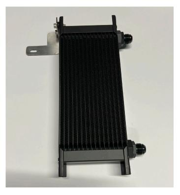
**4.** Remove the highlighted bolt and install the cooler bracket between the AC condenser and rubber grommet.
