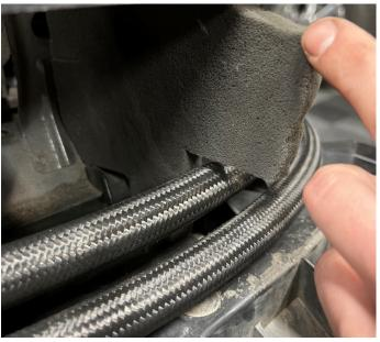
**12.** Find a suitable location and drill a 6mm hole in the plastic bumper support, using the supplied P-clip secure the hoses.
